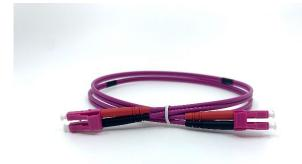
The duplex fiber patch cord is OM4 with 3 mm jacket. It is LSZH rated and its terminated with LC fiber optic connector on both ends.
